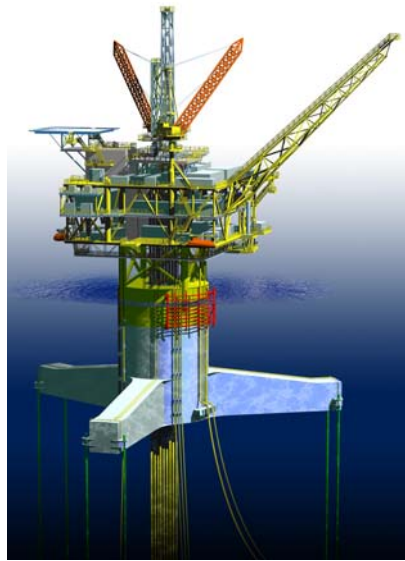
Figure 01: Principle of a TLP (the Atlantia Offshore Sea Star Design)
