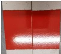
Formation of blisters was not observed and the delamination parameter were determined as “0” for all specimens confirming an excellent adhesion of the internal coating after the performed tests.
